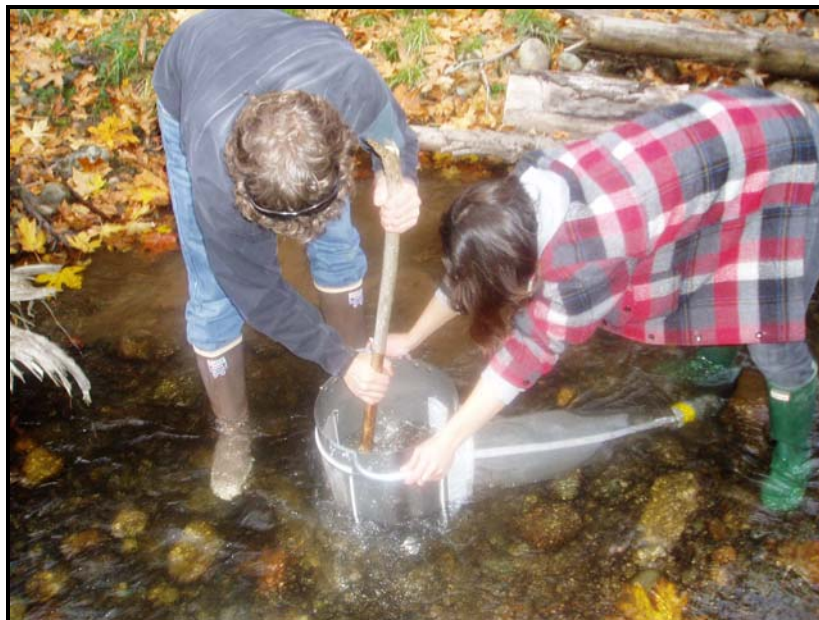
Photo 3. Melissa Colwell and Lukas Clarke obtaining a stream invertebrate sample with a Hess sampler at Station 3 located on the C.W. Young Channel.
