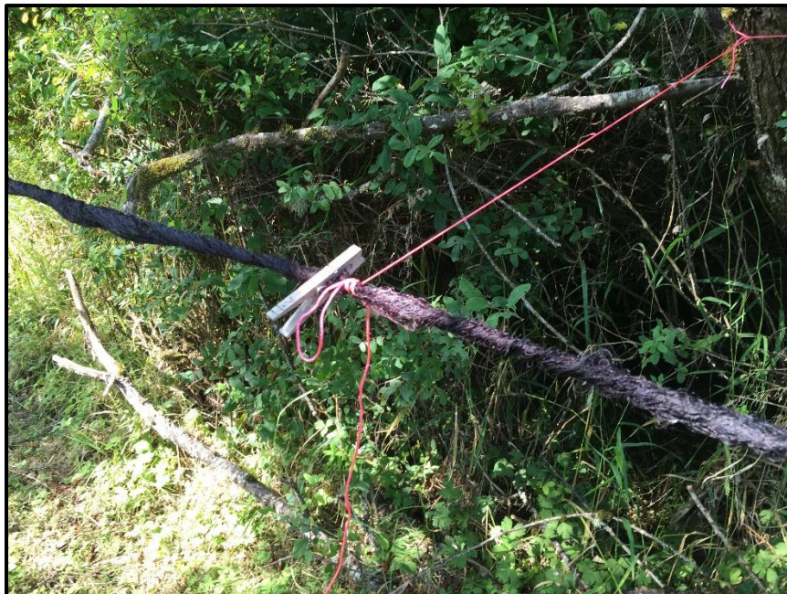
Photo F. Rope used to secure the middle of a closed and furling net. Note the slipknot and clothes peg.
