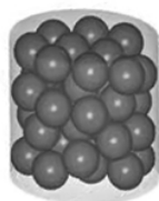
Figure 2: spheres packed randomly into a cylinder
