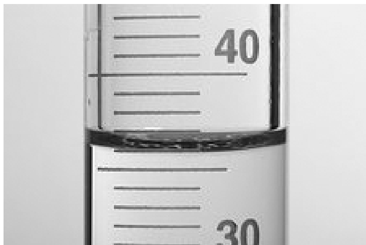
Figure 1: Reading a graduated cylinder
