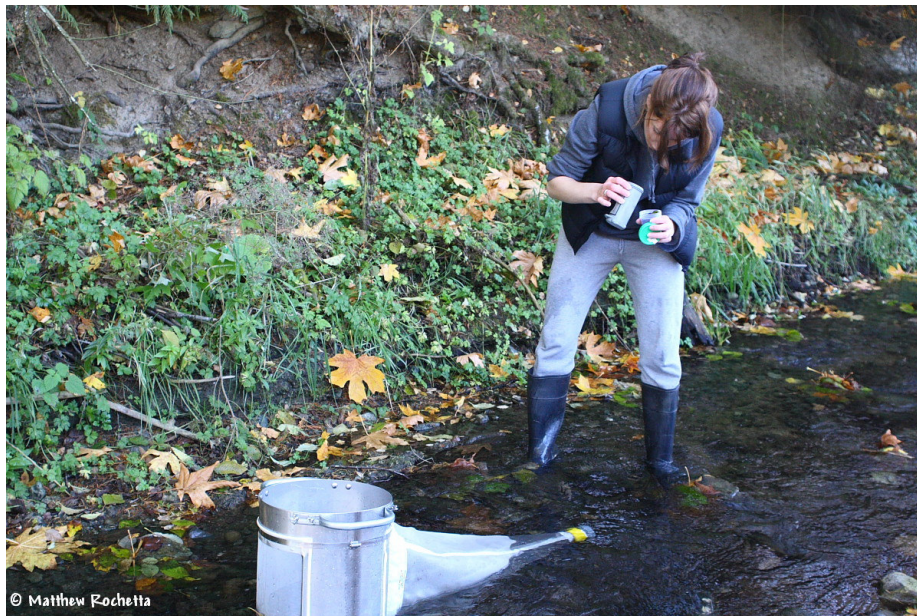
Photo 6. Laura Brown obtaining a stream invertebrate sample with a Hess sampler at Station 3.
