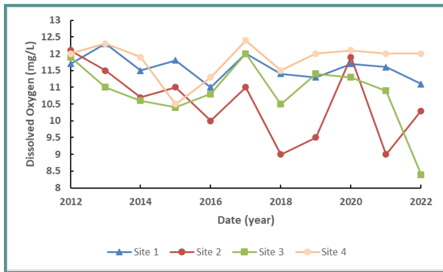
Figure 16. Temporal comparison of averaged dissolved oxygen concentrations (mg/L) at each site from 2012 to present.
