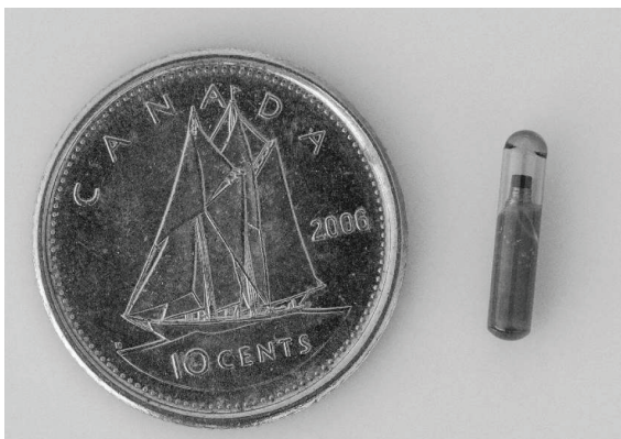
Fig. 4. Cyntag glass passive integrated transponder tag, 2 mm wide and 10 mm long, weighing 0.08 g.
