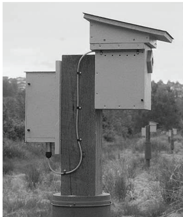
Fig. 2. Radio frequency identification datalogger box (left) and nest box (right) mounted to a 2.4 m length of wooden post. The two units are connected by a 26 American Wire Gauge magnet wire coiled around a plastic spool and inserted into the entrance hole of the nest box. Positioned around the post is a 0.6 m long cylinder made of 26 AWG galvanized steel ducting, functioning as a predator guard.
