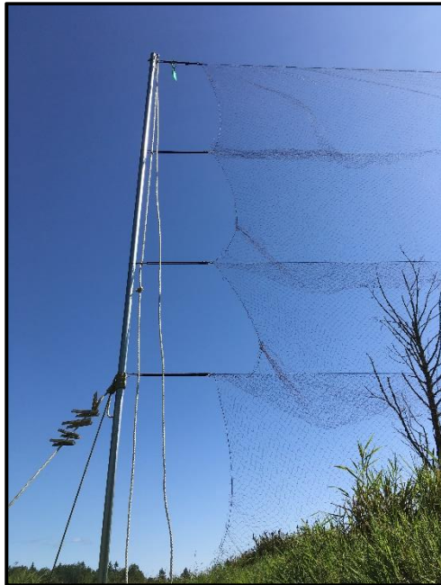
Photo D. Net pole and pulley rope assembly shown with a net open for capture. Note the net tag attached to the top trammel line loop.
